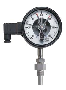
A glycerine filled indicator version is available as an option for service at measuring points exposed to strong vibrations. The fill dampens the measuring system when exposed to mechanical vibrations and thus enables steady indication; it also provides good lubrication for moving parts.
