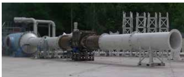
Flap valve test with INERIS notified body
