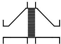
**Bi-directional in-line detonation flame arrester,
